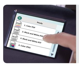
The Alaris S2000 Series Scanners allow for up to 20 tasks to be defined. Nine shortcut tasks are predefined but all can be easily customized to fit into your application needs. To add additional tasks to the pre-populated list, select the <NEW> option at the bottom of the Task Shortcut List.
